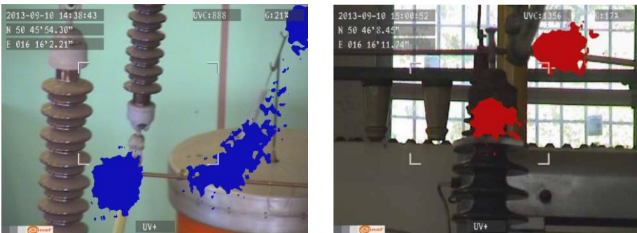
Fig. 3, 4. Corona discharge in laboratory conditions.
