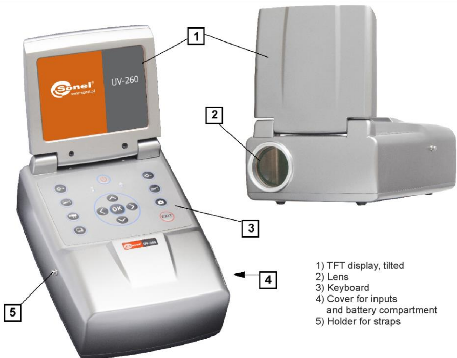
Fig. 11. Parts of Camera UV-260.
