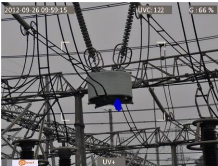
Fig. 5-8. Corona discharge in real power grids.
